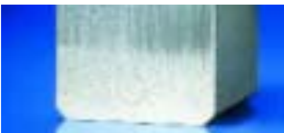
Ghostmarks, Difficult Commutation Causes: Commutation problems, such as false or incorrect position of the neutral zone or interpole
