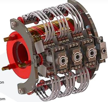
A carbon brush is not homogenous but pressed with a specific density that results in wear with small variations. To solve this, the V-Type is equipped with compensation rings for each individual carbon brush resulting in even wear of all brushes.
